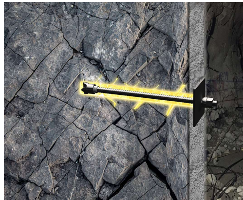
Rock Bolt Grout (RBG)
