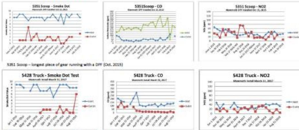
5428 Truck – DPF installed immediately following midlife engine rebuild (Mar. 2017)
