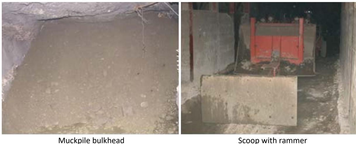
Figure 14 - Example of muckpile bulkhead.
