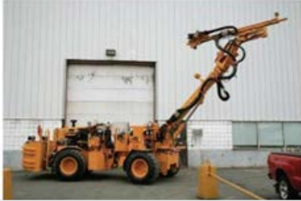
Figure 10 - A remote controlled drill for blockholing.
