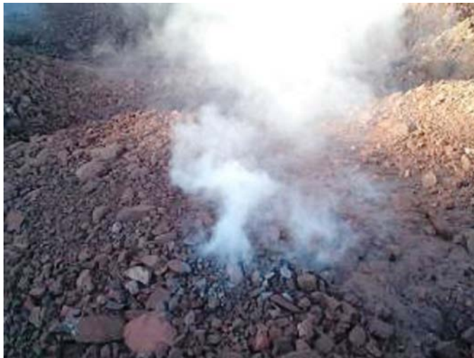
Figure 2 - Oxidation of broken ore.
