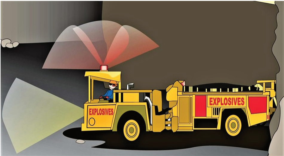
Figure 4 - Vehicle transporting explosives on surface shall have clearly visible explosive signage and red flag.
