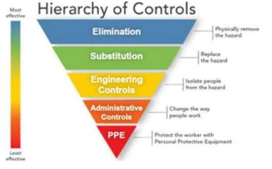
**Eliminating the hazard or substituting the process** by replacing diesel powered engines with electric or other types of power sources is the most effective strategy to eliminate worker exposure to DEE/DPM. The use of alternate fuels, such as biodiesel, is an example of substitution to reduce exposure, but potential risks introduced by alternative power sources or fuels must be taken into consideration.
