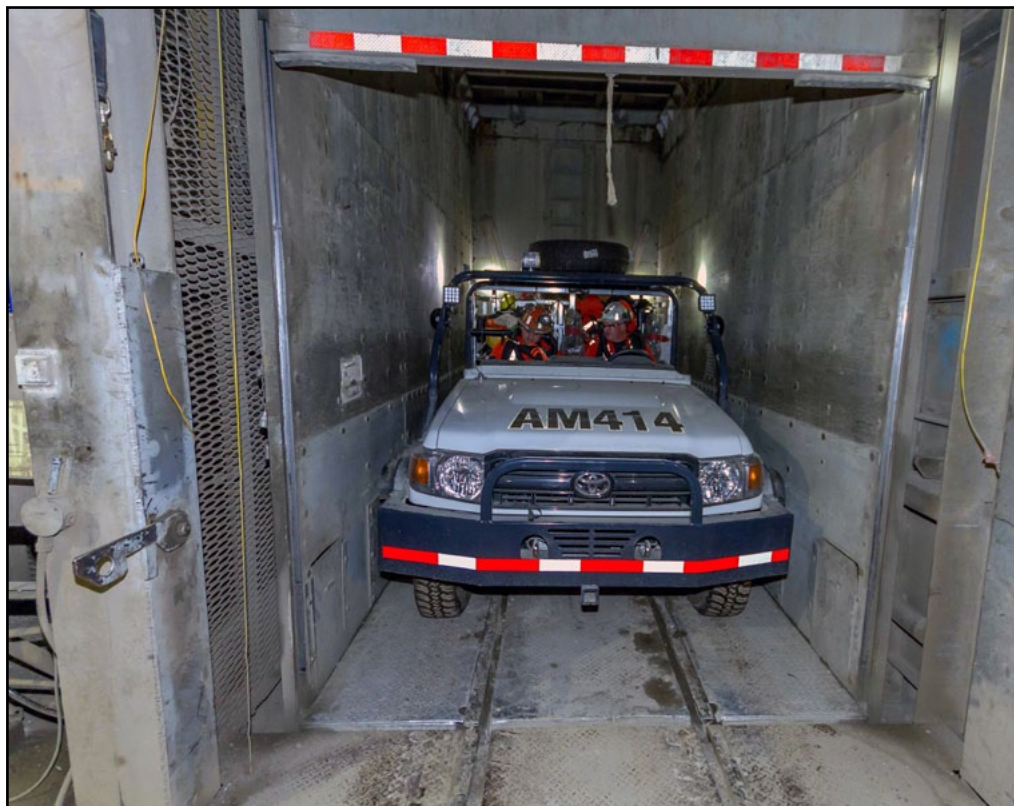
SOLVING THE PUZZLES – Fitting the Mine Rescue Emergency Response Vehicle (MRERV) on the cage at Kidd, keeping the stretcher in a horizontal position, and providing room for a six-man mine rescue team were among the design considerations Glencore’s Kidd Operations and Access Mining Services had to achieve in modifying a Toyota Land Cruiser.
